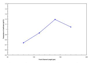
Figure 8: Drop volume temperature coefficient as a function of front channel length
