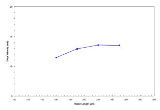
Figure 1: Drop velocity as a function of heater length at 32 °C
