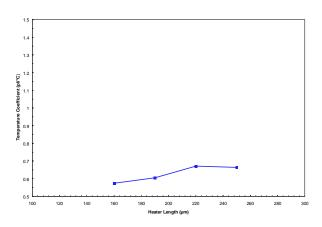
Figure 7: Drop volume temperature coefficient as a function of heater length
