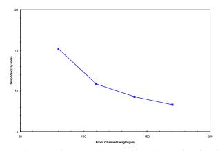
Figure 3: Drop velocity as a function of front channel length at 32  $^{\circ}C$
