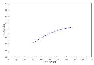
Figure 2: Drop volume as a function of heater length at 32 °C
